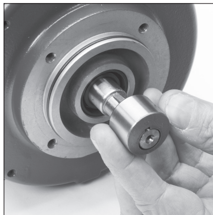
5.5 Remove and inspect cam (8) from motor shaft.
