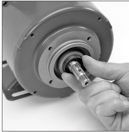
6.2 Lubricate and install shaft seal (10) onto motor flange with spring of seal facing pump.
