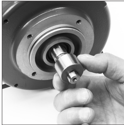
6.5 Lubricate and install cam (8) over motor shaft and key. Position cam (8) so stamped cam ID number is facing pump.
