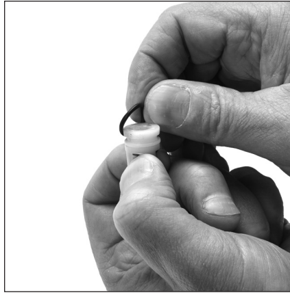
6.20 Lubricate and install o-ring (23) to seat (24). Repeat for second valve assembly.
