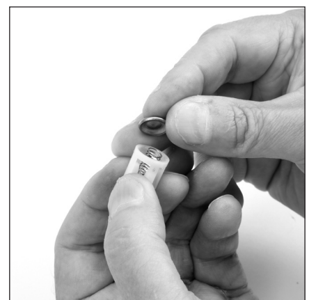
6.18 Place valve (25) cupped side over the spring (26).
