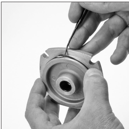
6.7 Lubricate and install o-ring (6) onto bearing cover (5).
