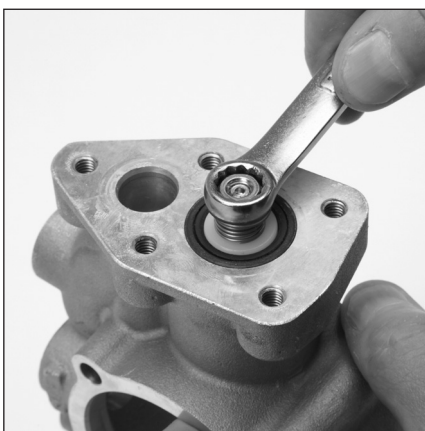
6.16 Apply Loctite®242® to M6 threads on plunger rod. Thread nut (16) onto M6 threads of plunger rod and torque to 25 in-lbs.
