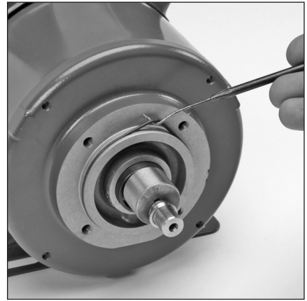
6.3 Lubricate and install o-ring (12) onto motor flange.
