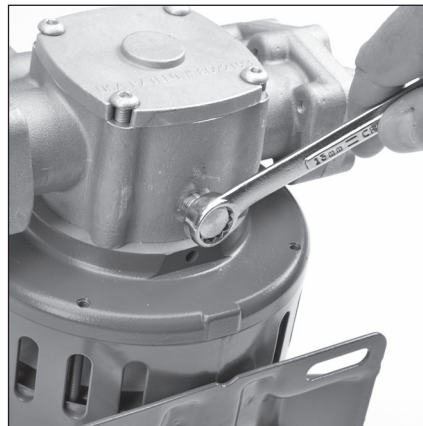
5.2 Use a 13mm wrench to remove brass drain plug (3) from pump crankcase (1) to drain water.
