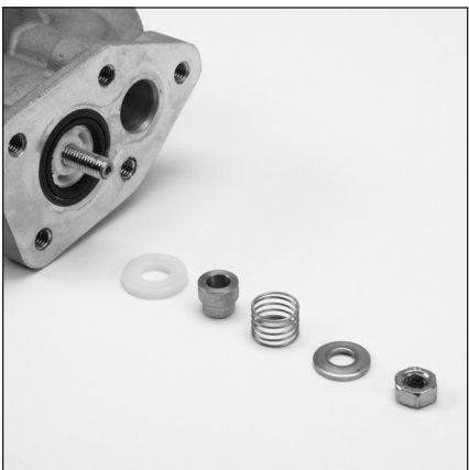
5.13 Remove and inspect nut (16), washer (17), spacer (19), spring (18) and inlet valve (20).
